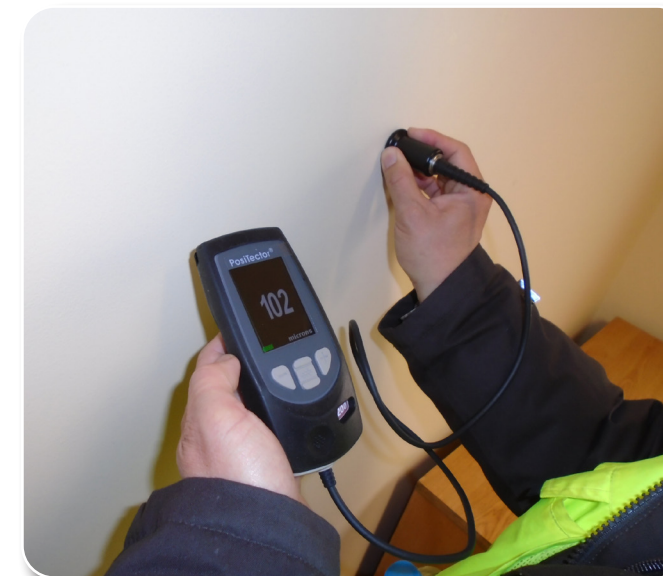
Construction Division's Quality Assurance Branch architect takes measurements of interior paint coatings to verify compliance with dry film thickness.
