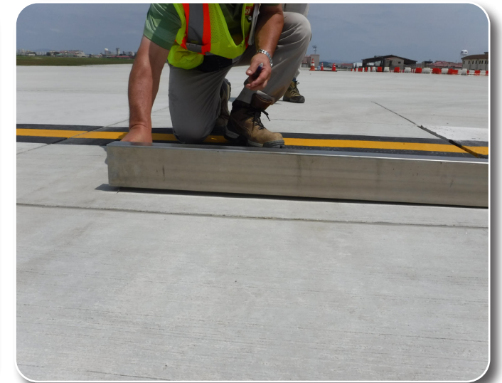
Construction Division's Quality Assurance Branch civil engineers check concrete surface smoothness on recently constructed airfield paving slabs using a straightedge.
