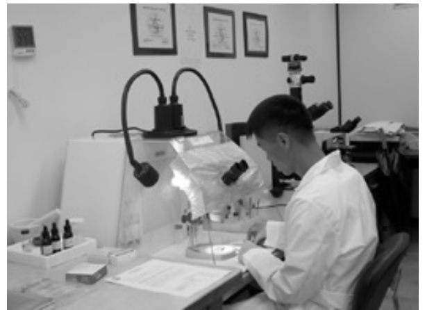
Mr. Park, Chong Pin, a laboratory analyst at the FED Asbestos Lab, prepares and mounts an asbestos bulk sample on a glass slide in a HEPA (High Efficiency Particulate Air) filter.
