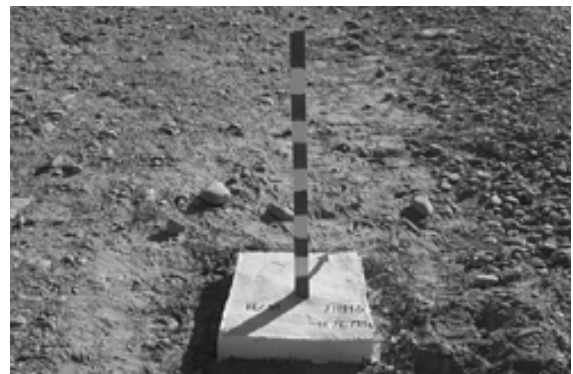
Minetech's benchmark with the azimuth and distance to the first corner monument for the cleared area.
