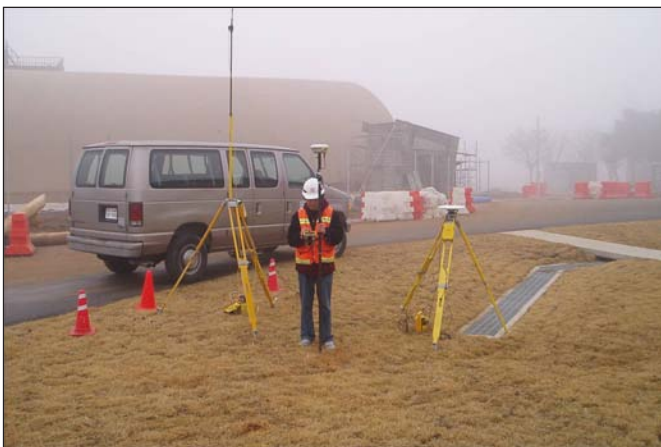
Landfill grade verification using GPS equipment at USAG Humphreys
