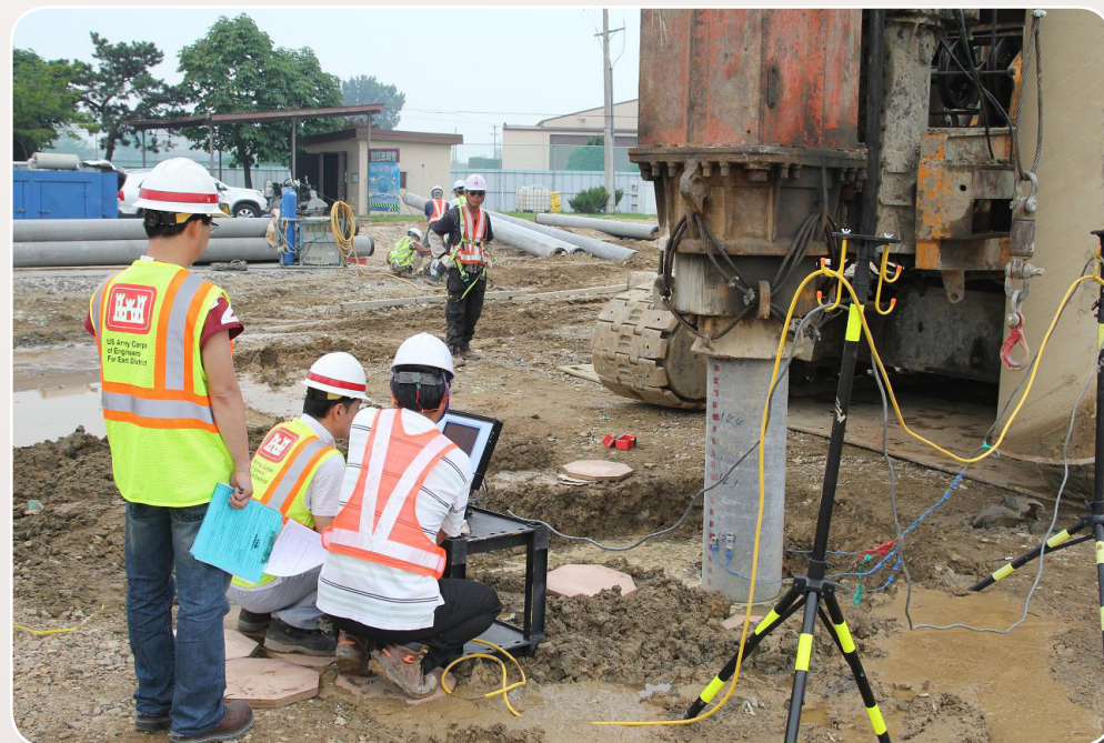
High-Strain Dynamic Testing of Deep Foundations. (FED file photo)
