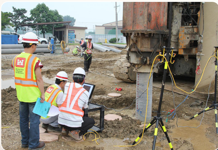
(above left) Soil Automated Consolidation Testing Equipment (above right) Soil Tri-axial Compression Testing Equipment (left) High-Strain Dynamic Testing of Deep Foundations (right) Soil Hydraulic Conductivity Testing Equipment (FED file photos)
