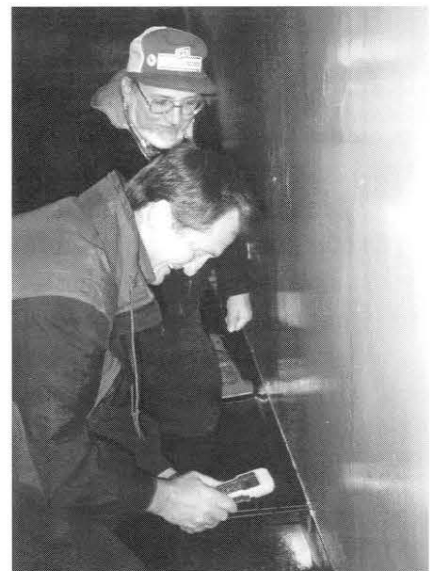
Mr. Vincent Hock (left), Principle Investigator, CERL, and Mr. Michael Connor, Chief Operating Officer, Dytronic, Inc., use a protometer to measure the humidity in the concrete walls and floors.
